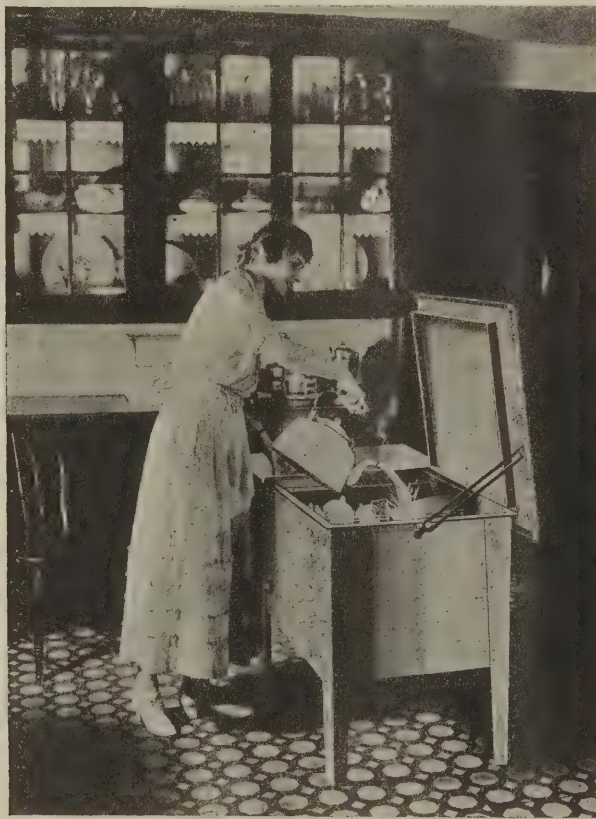
FIG. 1. AN ELECTRIC DISHWASHER FOR WHICH NO PLACE WAS PROVIDED IN PLANNING THE HOUSE. NOTE THE ADDITIONAL LABOR NECESSARY TO ITS OPERATION.
